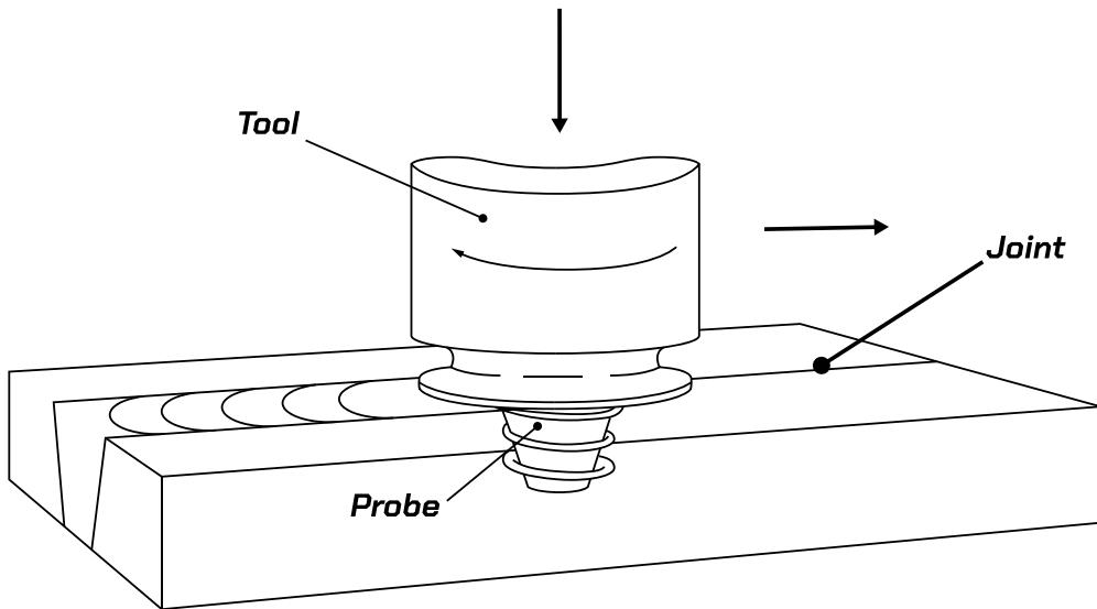
Friction Stir Welding (FSW) is often described as one of the most significant breakthroughs in metal joining since the invention of arc welding. Unlike traditional methods, it does not involve melting the material. Instead, it uses mechanical friction and pressure to “stir” two pieces of metal together in their solid state.
