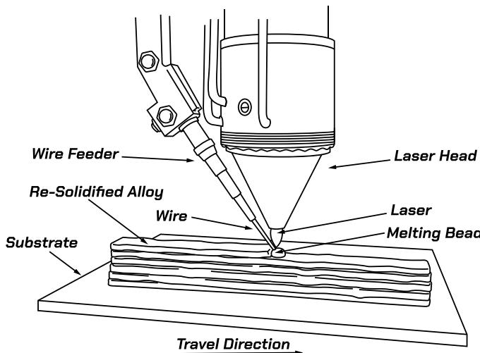
Wire Laser Metal 3D Printing is a technique that merges a high-power laser with a continuously fed wire to create near-net-shape metallic parts. Unlike powder-bed fusion, which relies on fine powders, this method uses wire as feedstock, ensuring a safer and cleaner process. The wire is melted by the focused laser and deposited layer by layer along a programmed path, producing dense, structurally sound components.
