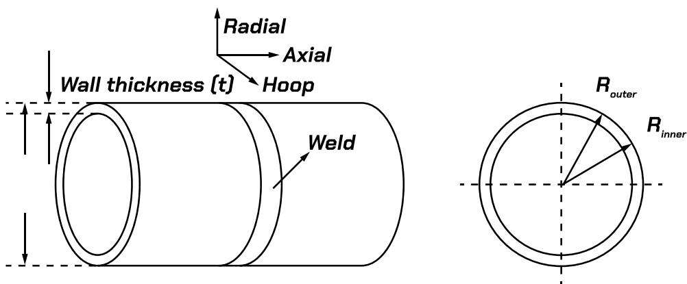
Residual stresses are an unavoidable byproduct of welding, created when rapid heating and cooling cycles cause uneven expansion and contraction of the material. These hidden stresses can distort parts, shorten fatigue life, or even trigger premature failure in safety-critical structures. **Smart prediction of residual stresses** seeks to address this challenge by integrating computational models, sensor systems, and artificial intelligence into the welding process.
